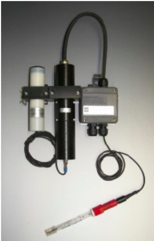
ORI MODULE with METTLER TOLEDO InPro3250i SG pH electrode
