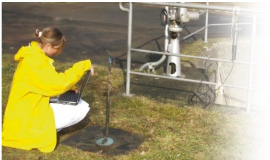
Engineer accesses an ORI MODULE via a wireless connection
