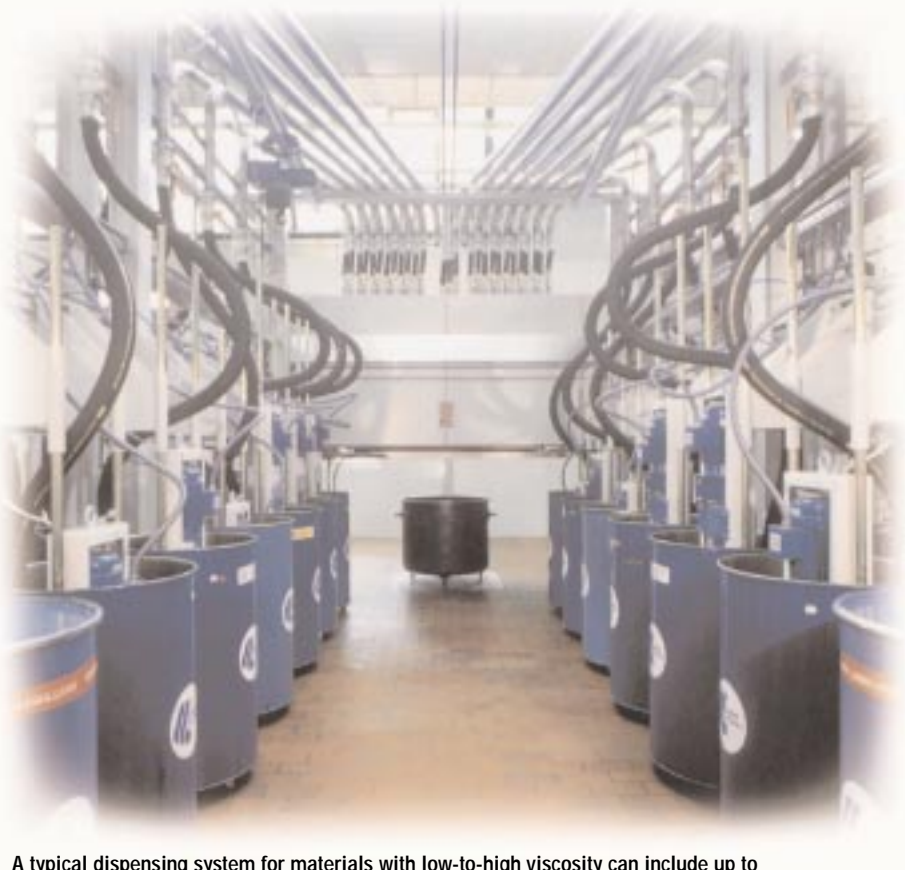
A typical dispensing system for materials with low-to-high viscosity can include up to four scales.
