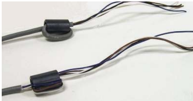
Figure 2-11: Installing the Ferrite Cores
