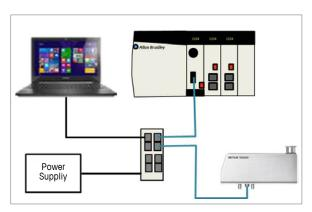
For a network connection to an Allen-Bradley PLC via EtherNet/IP network, you need an IEEE 802.3af Power-over-Ethernet switch to provide power to the weigh module.
