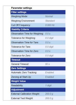
The webserver identifies the individual weigh module configuration including type, software version, IP-Address but also specifications and weighing parameters. It is also possible to show the weight value.
