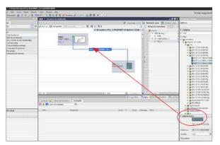
After installation of the GSDML file, the WMF weigh module is available in the hardware catalog. It can be added to the project by dragging and dropping the file.
