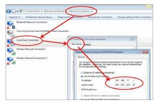
The IP address for establishing connectivity with the computer can be set as shown in the following pictures. The computer and Weigh Module must be in the same IP-Address range. The default IP-Address of the Weigh Module is192.168.0.55.
