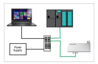
Network for connecting to a Siemens PLC over TIA Portal or Simatic Step 7 Manager via PROFINET IO requires an IEEE 802.3af Power-over-Ethernet switch to provide power to the weigh module.
