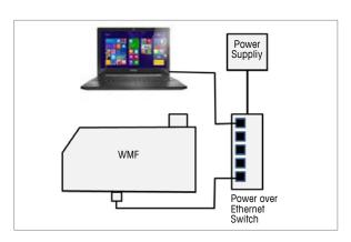
The configuration of the weigh module can be checked from the webserver. Connect the weigh module to a computer via a Power-over-Ethernet Switch using an RJ45/M12 patch cable. Enter the weigh module's IP address (default: 192.168.0.55) into the computer's browser.
