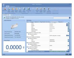
You can configure the IP settings of the weigh module using APW LinkTM PC configuration software. You can download this software from www.mt.com/apw-link
