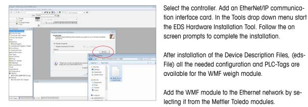
Use the fixed IP address which was set with APW-Link. [Note: DHCP should not be used in control networks.] The number then must be transferred manually into the weigh-module setting.
