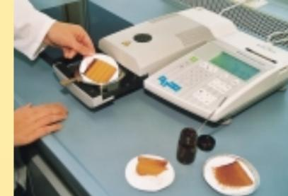
Samples are prepared using a special spatula: a fine coating is spread on a round heat resistant fibreglass paper
