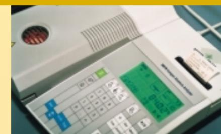
A protocol is printed out while the drying is in progress. The HR73 halogen moisture analyser provides TAKASAGO Europe with important results for process control within minutes
