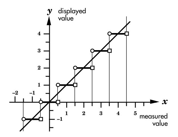
Limiting the displayed value to one display step introduces the following quantization error:
