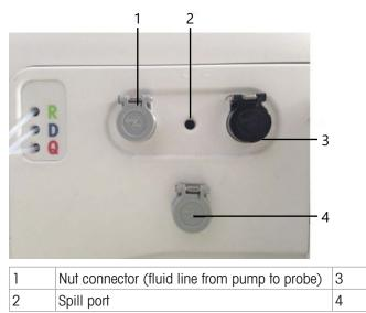
Nut connector (fluid line from probe to needle)
