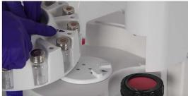
4 Rotate the rack lever clockwise to lock it in place.
