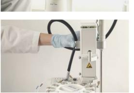
2 Fix the needle in place with the knurled screw.
