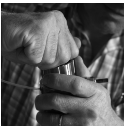
Fig. 6: Screwing on the new MembraCap
