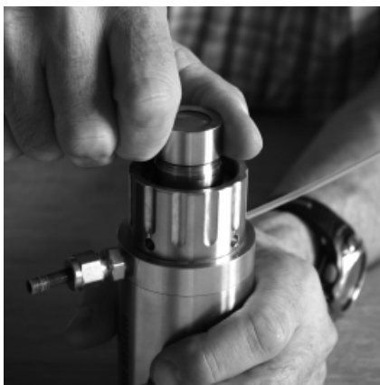
Fig 4: Unscrewing MembraCap counterclockwise
